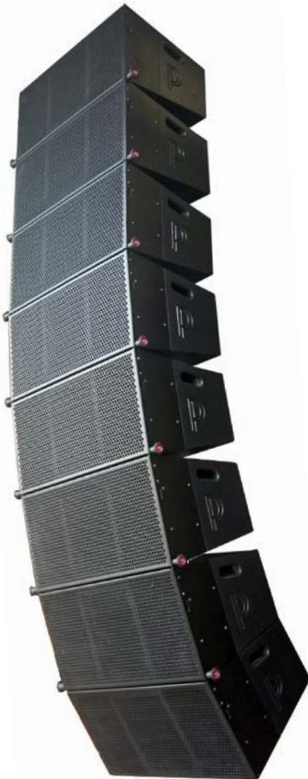
**The PLA21021** is a 2-way true line source enclosure, with a controlled dispersion pattern of  $110^{\circ} \times 15^{\circ}$ , using advanced waveguides for the  $2 \times 1"$  Neodymium drivers, and  $110^{\circ}$  soundguides for the two High-power neodymium  $10"$  woofers, controlled dispersion is achieved over a very impressive frequency range.
