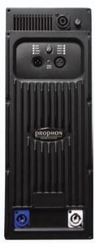
Picture showing the active module with Neutrik powercon in/out, Neutrik XLR in / through, Speakon out to either a passive B1HP to drive it as a slave, or to a passive fullrange speaker to be used as a top in an active sound system.
