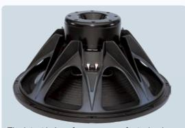
The latest in Low frequency woofer technology, with external cooling system, ventilated and double wired voice coils, double spiders
