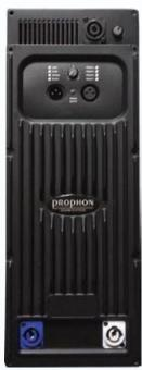
Picture showing the active module with Neutrik powercon in/out, Neutrik XLR in / through, Speakon out to either a passive B4HP to drive it as a slave, or to a passive fullrange speaker to be used as a top in an active sound system.
